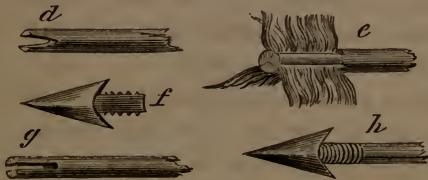
d , arrow nock ; e , section of arrow, through feather ; f , steel arrow-head ; g , slit in shaft to receive head ; h , head wired on.
